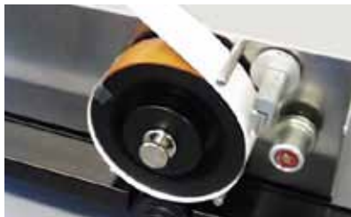
Mounting substrate for gravure
