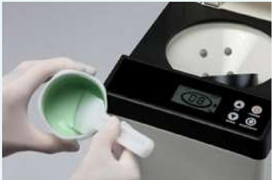
The typical mixing time for fully dispersing a powdered pigment into a silicone sealant, or mixing a fumed silica or precipitated chalk silicone formulations is less than 20 s. These are all operations that would otherwise require three hours or more of mixing time. Additionally, the spinning action of the mixer removes air from the blend, yielding a finished product when the mixing process is done.
